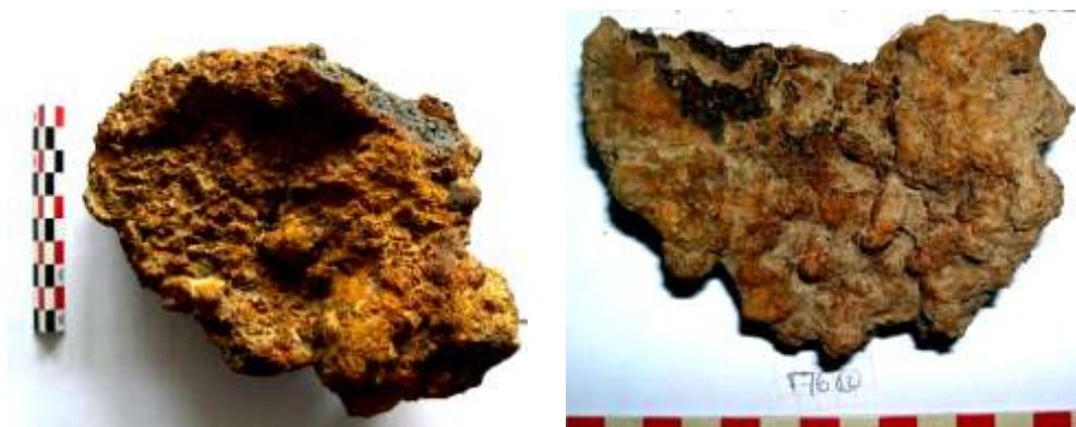
Figure 29 : Scories plano-convexes de forge
